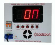
Pressing to ON button starts the water pump and the LED indicates this with the word ON
