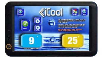
temperature you require by simply touching the up and down arrow buttons. As you make changes the new pool water temperature setting will appear on the screen in a blue window marked "Selected Temperature". The right-hand side of this screen shows the outside air Temperature.
